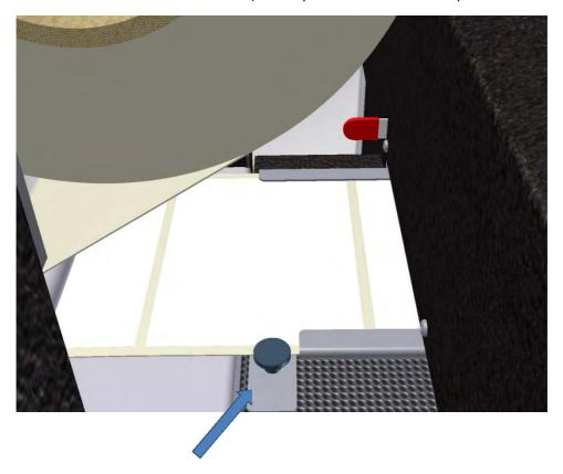
Press the "Load / Unload" button. The printer will start to pull in the labels and feed them up to the print position. The tension of the label stock indicates that the label stock has been successfully loaded. The printer is now ready for operation.
