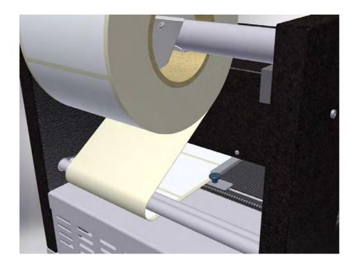
Move the adjustable label guide on the right up to the label stock and secure the guide with the **screw**. The label guides should hold the label stock securely without squashing the liner. The labels should move through the feeder easily and without creasing.
