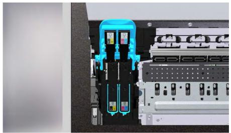
Lower the print head release lever and close the printer cover.
