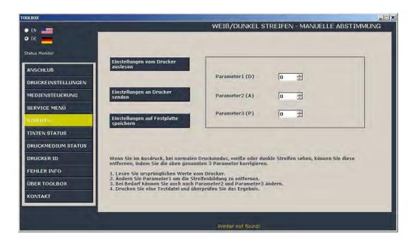
You can correct white or dark lines on the printout in normal print mode by adjusting the three above parameters.
